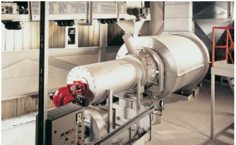
Triplex dryer with hot gas generator
