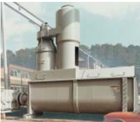
lime hydrator with wet scrubber
